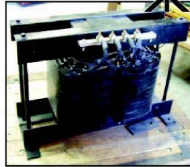
Current Limiting Reactor
